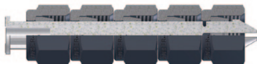
Cross-section of an arbor with five nut ferrule sets
